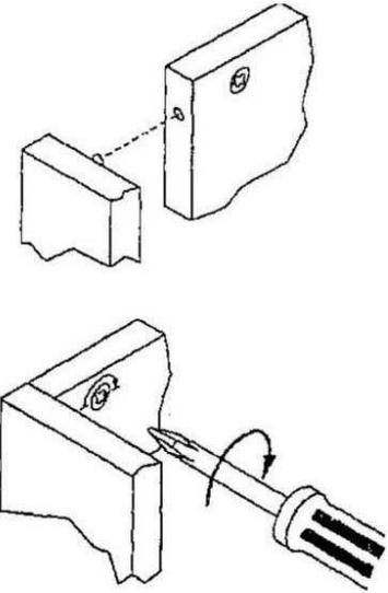
Fasten panels together and make sure all cams are locked.
