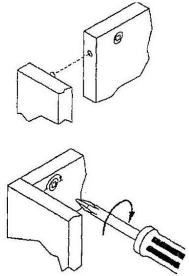
Fasten panels together and make sure all cams are locked.
